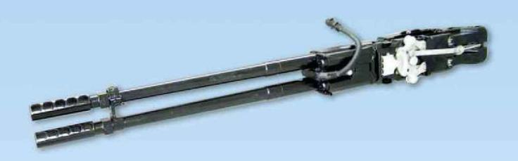
I USE: The two-barrel cal. 23 x 115 mm air to air cannon is designed to be mounted on aircraft fighter. It is intended for air defense and against ground targets.
